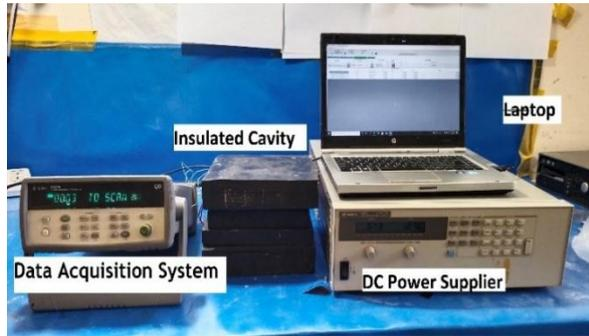
**Figure 2: Actual Experimental Setup**
