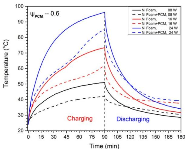
Figure 5: Temperature comparison for different heat sink configurations.
