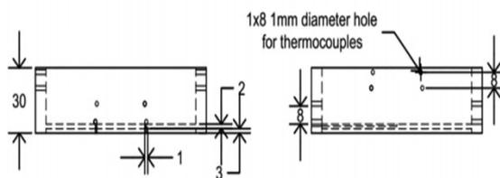
**Figure 3: Thermocouple placement diagram.**
